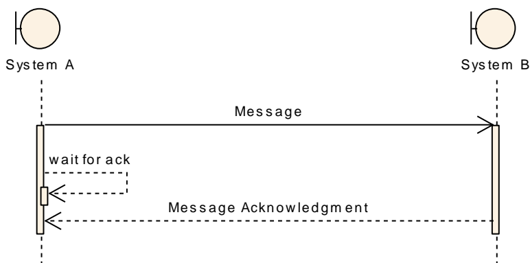
Figure 2.3.2.1. Successful Message Exchange Sequence Diagram
